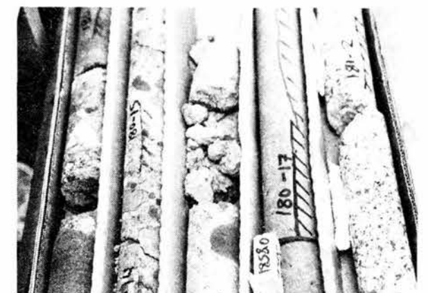
CORE SAMPLE segments detail an encounter with a magma conduit — (from left) three breccia segments, a rhyolite, and a granite.
